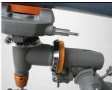
obr. 2-15 obr. 2-16 Hriadeľ R.A. - dole a hriadeľ DEC. - hore
